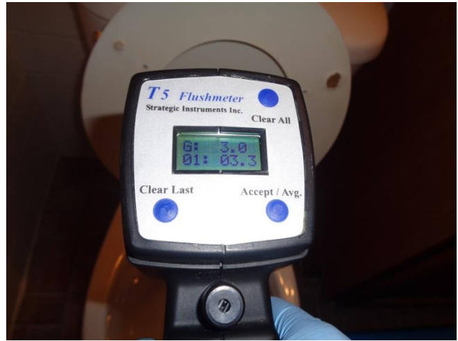
Figure 29: Typical Test Result for Toilet Flush Test
